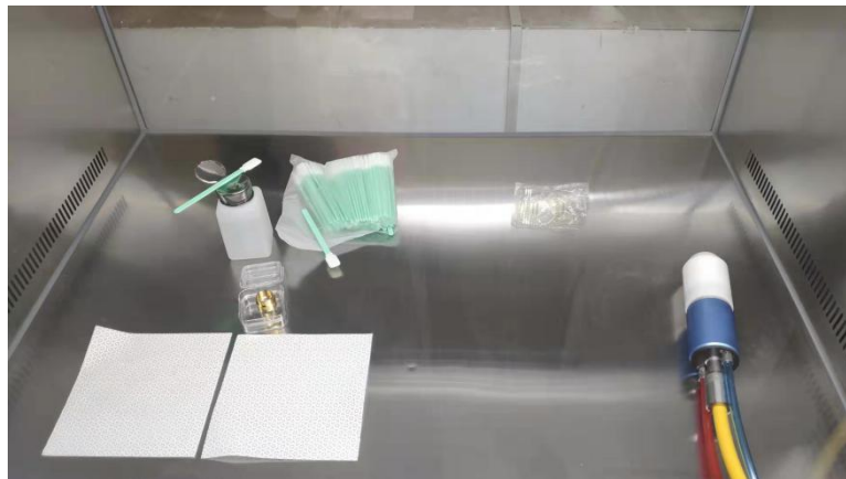
Figure 6 output optical cable placed in cleaning workbench and with air extraction.
