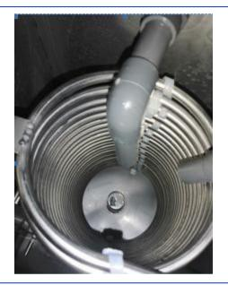
After opening the top of the tank, you will see the suction filter at the bottom of the tank (as shown in the picture above).
