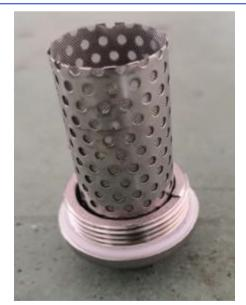
Use an air gun to clean the dirt and impurities filter
