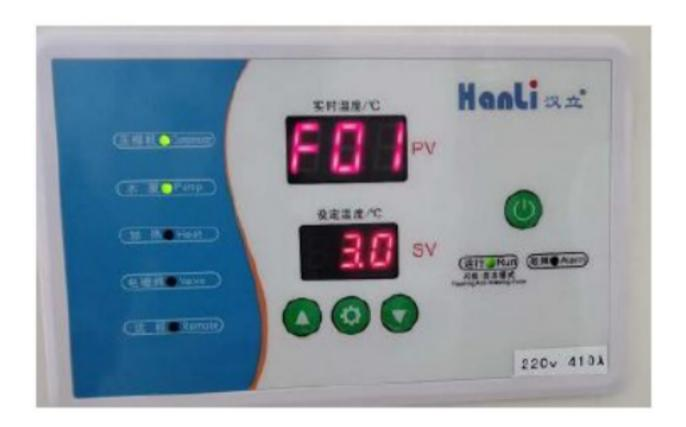
Press setting button to enter the setting, Press the up and down button to adjust the set value, After pressing the set button to confirm the save, press the power button to exitGenerally, the default production settings are as followed:
