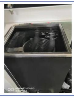
Open the side door of the chiller, and you will see the water filling tank of the equipment as shown in the picture below
